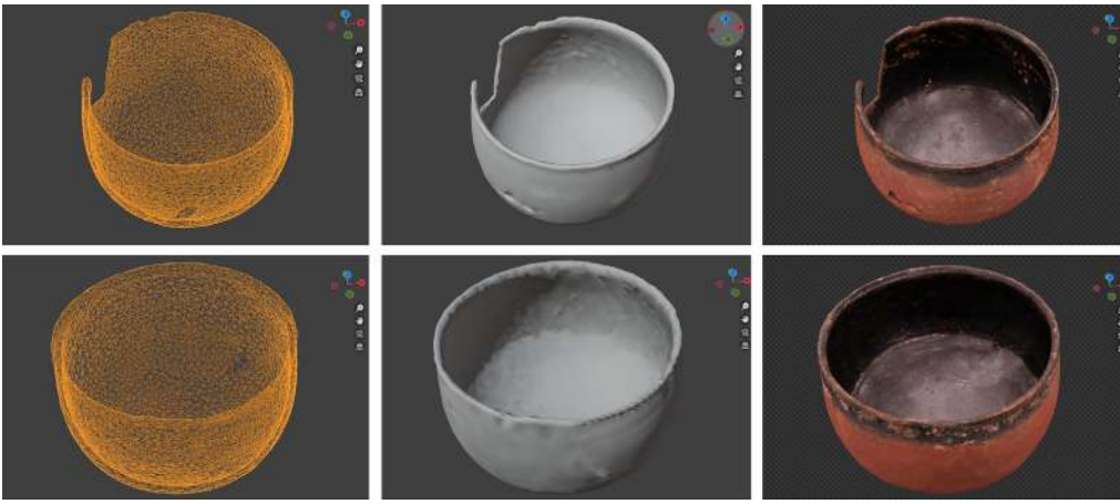
Image 2: Textures and details from the high-poly model were baked onto the low-poly version. Blender tools were used to address gaps and restore missing parts with final touches made to model's texture.
